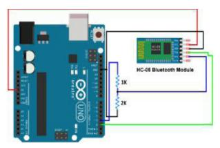
Figure 5: HC-05 Bluetooth Interfacing with Arduino UNO
