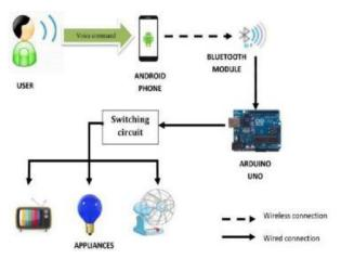
Figure 1: Block Diagram of the proposed System
